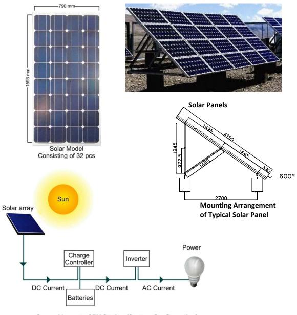
General Layout of PV Station (System Configuration)
